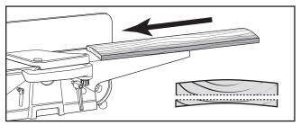
**2. Surface Plane On a Thickness Planer**—The opposite face of the workpiece is surface planed flat with a thickness planer.
